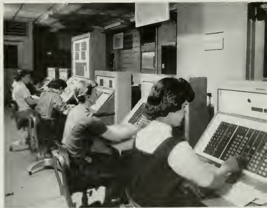
8. All of Bizmac's 220 units can be operated by remote control from this room, known as System Central, which is similar to a telephone exchange.
